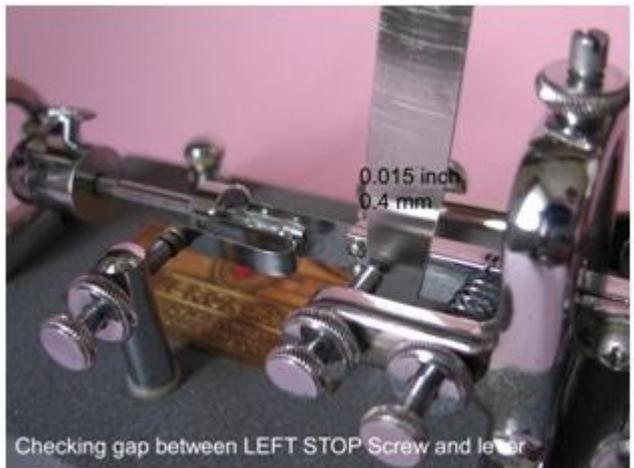
*Checking gap between left stop screw and lever*
