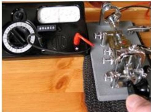
*Checking the dot contact spacing*
