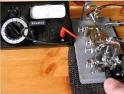
*Checking the dot contact spacing*
