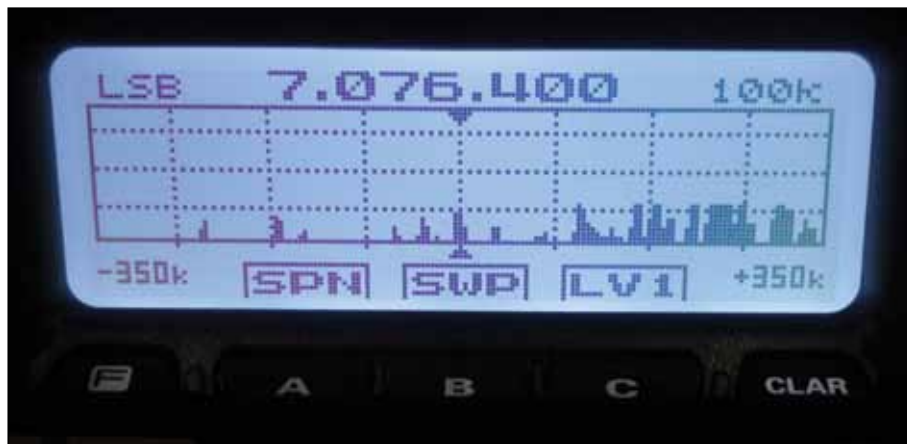
Fig. 1: The spectrum display is handy and remarkably clear given the screen size.
